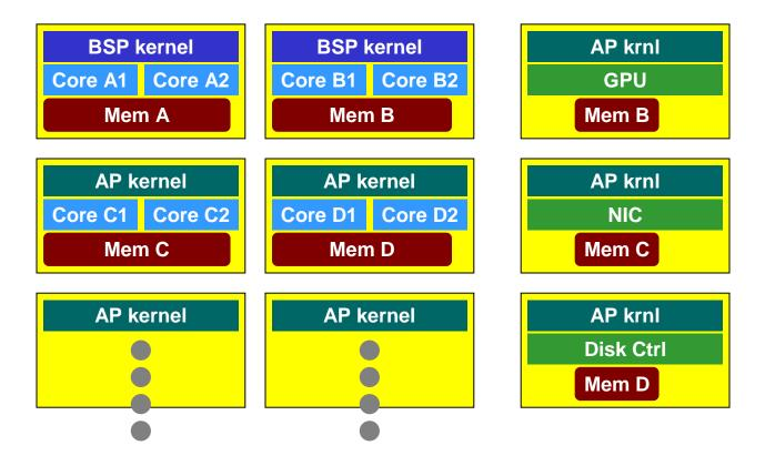
The left part of the figure basically shows the NUMA nodes (internal processors), while the right part of the figure shows the external processors such as the GPU, NC, and Disk Controller. Each NUMA node in
